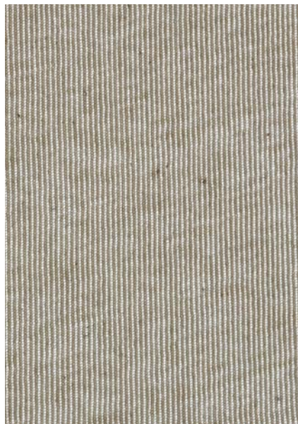
Fig. 19: With 100% cotton, the best evenness was achieved using the classical process.
