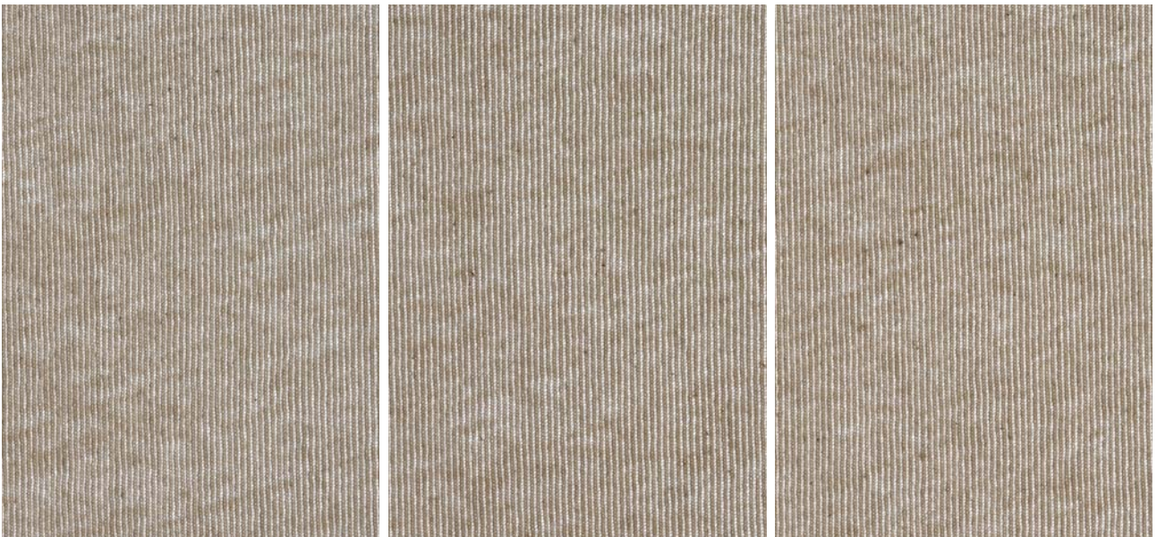
Fig. 21: With 30% cotton and 70% noil, a clear difference in favor of the direct process can be seen.
