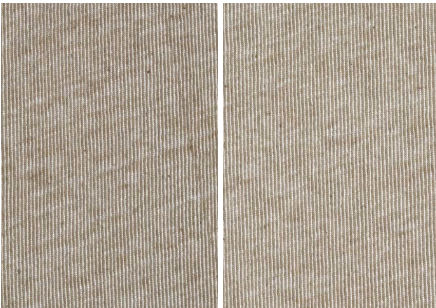
Fig. 23: Comparing the direct process with one or two draft zones, the one with two draft zones produces the fabric with a better evenness.
